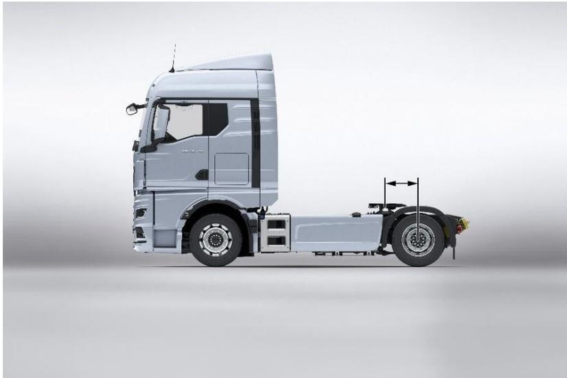
The fifth-wheel lead is the distance measured (in millimetres) between the middle of the last axle and the middle of the kingpin when coupled. This applies irrespective of the total number of axles with which the vehicle is equipped and whether the last axle is driven or not - in other words, it also applies to vehicles with a trailing axle.
