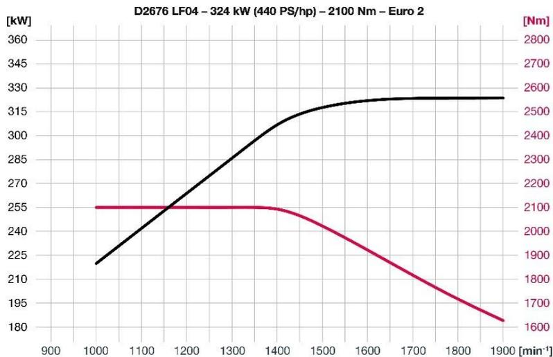
With 440 hp (324 kW) and 2,100 Nm max. torque, the MAN D26 Euro 2 engine offers reliable, economical and powerful propulsion. A high-torque performance characteristic with extremely economical fuel consumption distinguishes this 12.4-litre six-cylinder in-line engine with Common-Rail injection.
